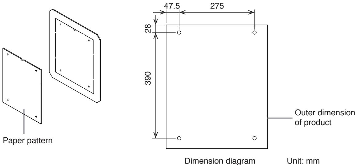
**Step 3.** Installation dynabolt/anchor sleeve size 10 ( This is not supplied with product)
