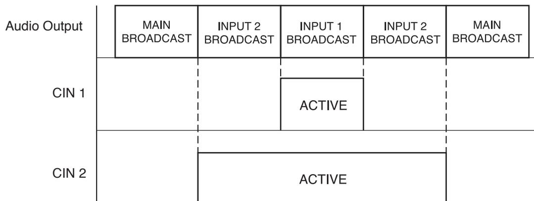
The priority level will be INPUT 1 >> INPUT 2 >> MAIN BROADCAST (FRONT MIC and Optional MP3 Player module). To activate audio signal from INPUT 1 and INPUT 2, need to triggering CIN 1 and CIN 2.
