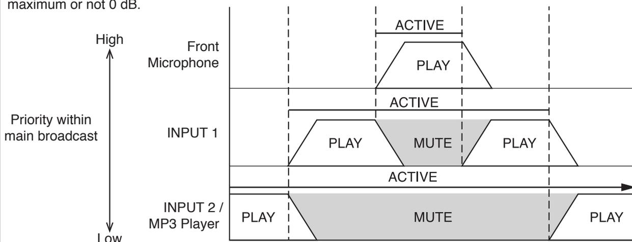
The priority level will be FRONT MIC >> INPUT 1 >> MAIN BROADCAST (FRONT MIC and Optional MP3 Player module). Priority level triggering by signal audio from Front MIC and INPUT 2.
