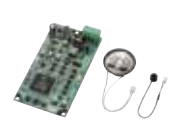
Door Station Board
